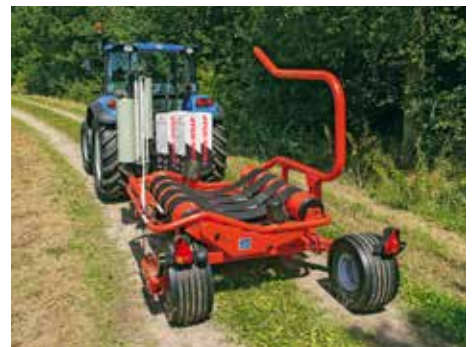
Limited transport width due to adjustable wheel positions
