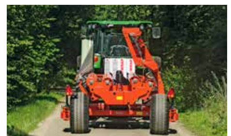
For road transport the wheels can be folded inwards to reduce the transport width. Hydraulic folding is optional
