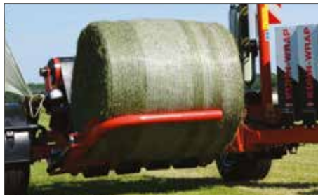
Quick and gentle loading of the bale guaranteed with the long loading arm
