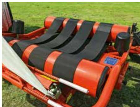
Four evenly wide-spaced endless belts
