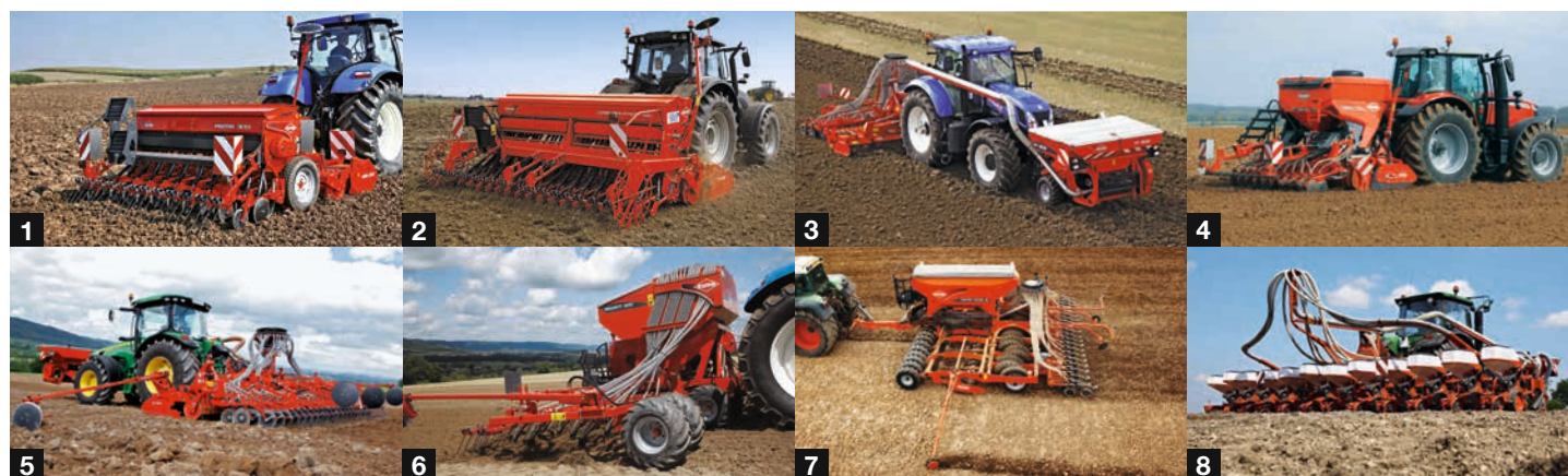
1. mounted mechanical - 2. integrated mechanical - 3. with front hopper - 4. integrated pneumatic - 5. mounted seeding combinations - 6. mounted for min-till seeding - 7. trailed for min-till seeding - 8. precision seed drills
