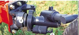
**TRANSPORT WHEEL WITH SUSPENSION** The plough can be transported on the road in complete safety thanks to a 540mm diameter transport wheel equipped with its own suspension system **4** serving to protect the plough and tractor from possible transport shocks. The wheel can be swung into the transport position in a single movement by pulling on the locking pin. **5**.
