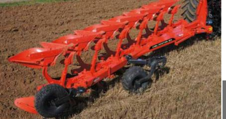
The wheel is equipped with a central pivot allowing it to automatically follow any changes in working width. The
