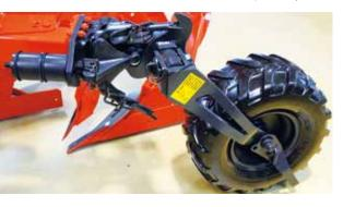
**COMBINED WHEEL** a single wheel ensures both work and transport positions
